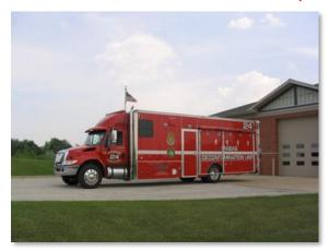
Mass decontamination – up to 200 people with supplies on board. Shower and hygiene facilities. Exterior, under-awning, misting nozzles for cooling or mass decontamination.
