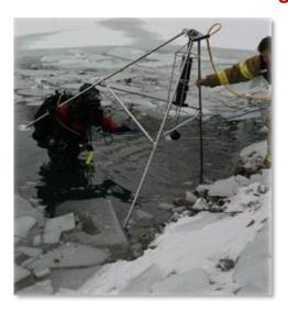
The sector scan HD sonar head is deployed to the bottom on a tripod. The system is operated from a laptop computer and high-resolution images are produced as the unit scans in a 360° view. Scanning results allow real time conditions that provide diver coordination and maximizes diver safety in order to fulfill rescue and recovery operations.
